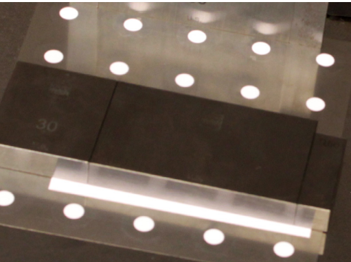
Perspective image corrected for lens imperfections. Straight lines appear straight.
