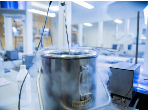
Calibration using liquid nitrogen up to -90\text{ }^{\circ}\text{C} .
