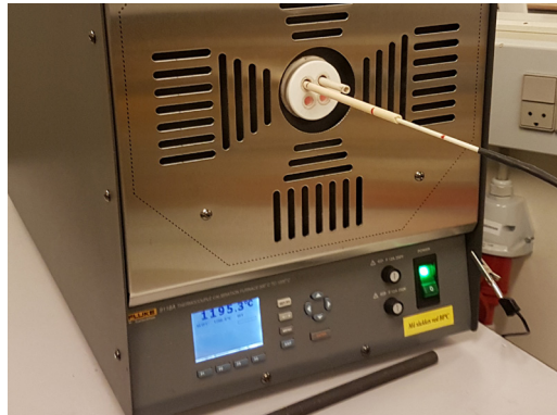
Calibration of thermocouples up to 1600\text{ }^{\circ}\text{C} .
