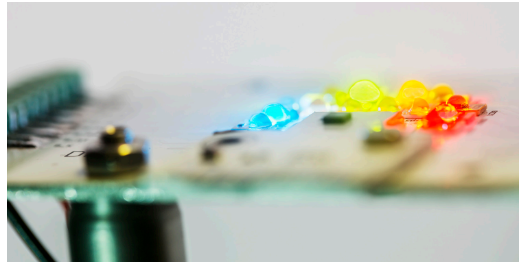
Multi LED board for color testing and source optimization.
