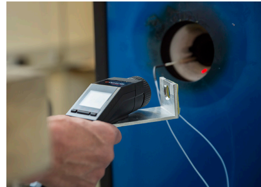
Non-contact temperature sensors calibrations using black bodies.
